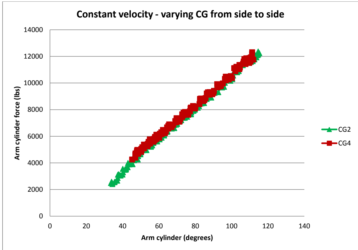
Figure 26: The force results of the arm cylinder were measured at medium weight (3,300 pounds) for the two lateral CG locations.
